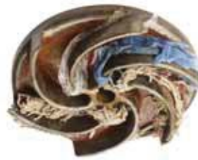
Figure 6: Accumulation in a vortex impeller
