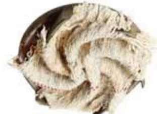
Figure 7: Accumulation in a vortex impeller
