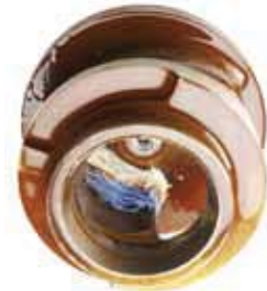
Figure 5: Accumulation in a single-vane impeller
