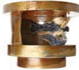
Figure 4: Accumulation in a single-vane impeller
